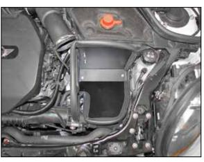
12. Install the heat shield into the vehicle so the mounting studs engage the mounting grommets and then secure the heat shield with the battery cover bolt removed in the previous step.
