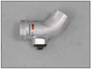
14. Install the mass air sensor into the K&N<sup>®</sup> intake tube and secure with the provided hardware.
