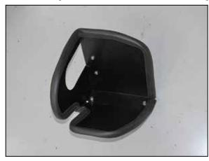
9. Install the 56" edge trim around the heat shield as shown.
