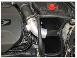
15. Install the K&N<sup>®</sup> intake tube into the heat shield and turbo inlet hose and then secure the tube with the provided hose clamp
