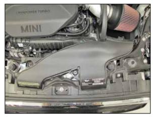
18. Reinstall the fresh air intake scoop and secure with the factory hardware.
